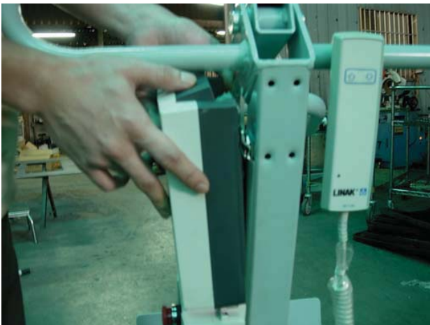
Fit battery onto control box.
