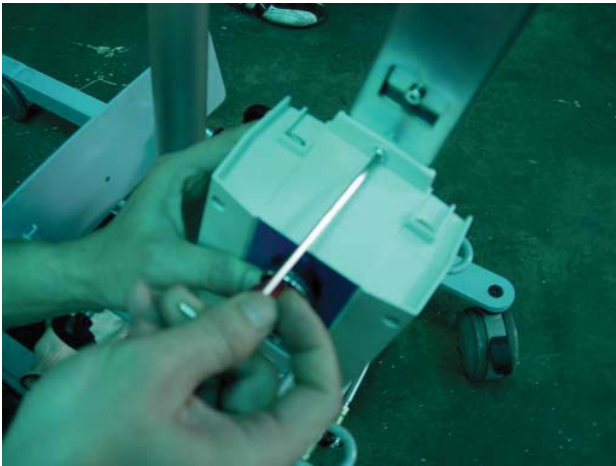
Tight up control box.
