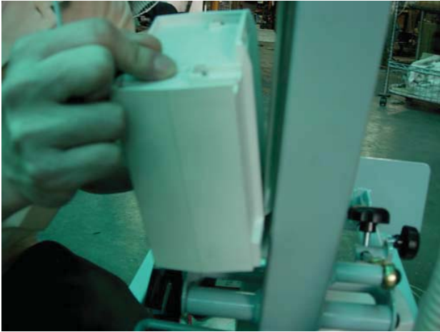
Fit control box onto bracket (on mast).
