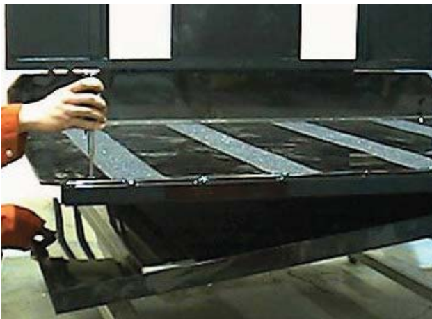
FIG. 7A- LOWER SAFTEY PAN TO ACCESS BOLT HOLES
