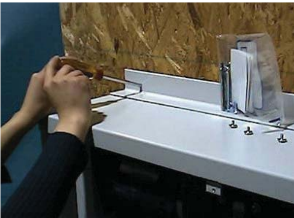
FIG. 21- MOUNT TOWER TO EXISTING STRUCTURE
