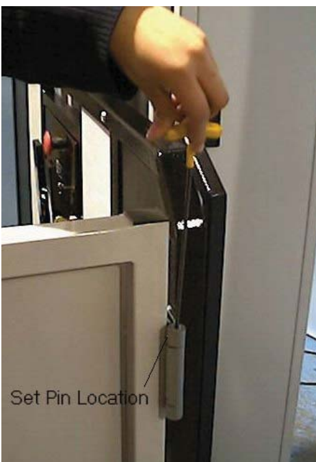
FIG. 13- ADJUSTING SPRING LOADED HINGE
