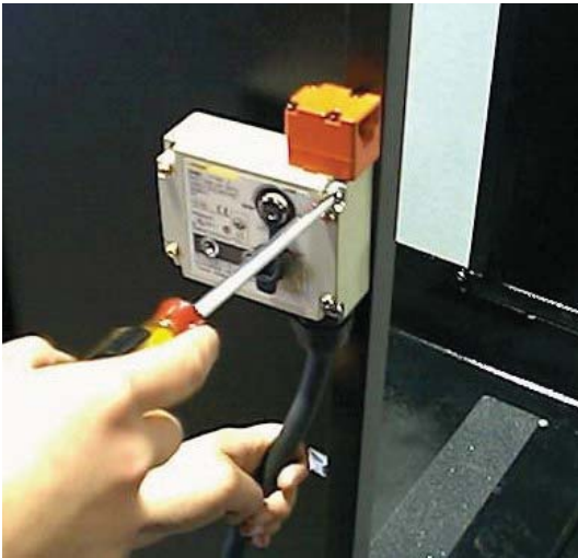
FIG. 11- MOUNT INTERLOCK TO SOLID HANDRAIL
