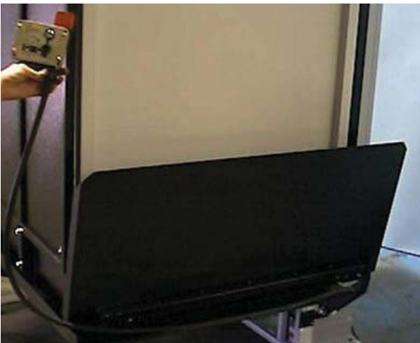
FIG. 10- RUN CABLE UNDER TOE PLATE
