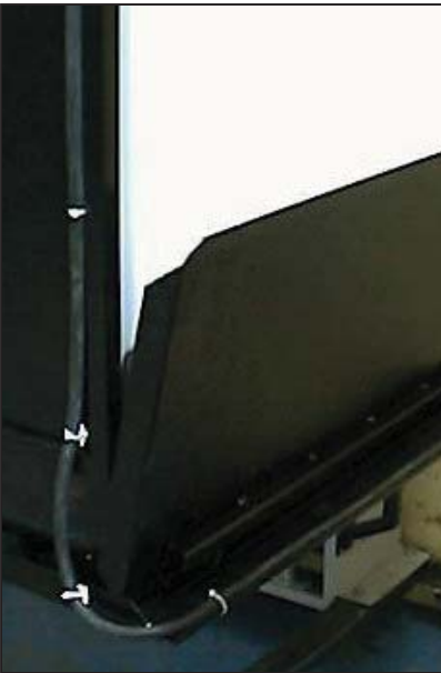
FIG. 14- FASTEN CABLE TO SAFETY PLATE USING STRAPS
